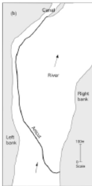
Figure 1 Irregularly shaped traditional anicut. Scale in meters.
